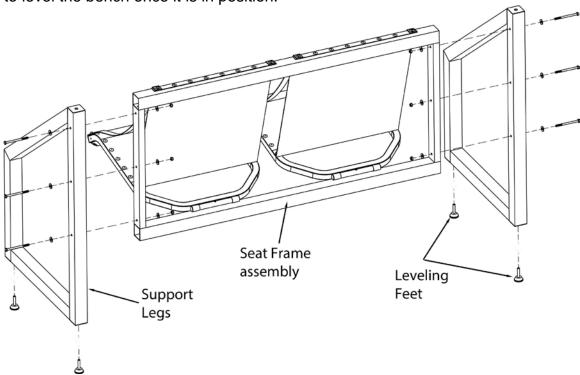
Note: Millennium products are manufactured using very tight tolerances so it may be necessary to tap the bolts into the holes with a hammer, this is normal and makes for a much quieter product.
